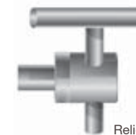
Backpressure valve on tee for pressure relief
